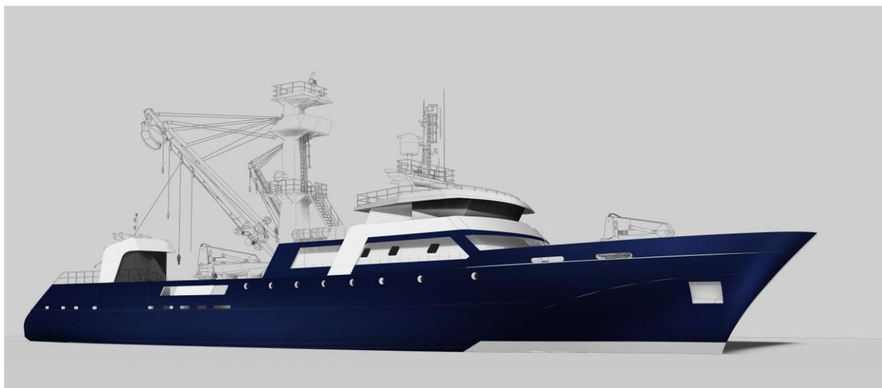
SAUPIQUET has just confirmed to PIRIOU the order of a 67m tuna seiner dedicated to oceanic tuna fishing. This new unit to be delivered by the end of 2020 will be built by PIRIOU Vietnamese shipyard, which has already built and delivered eight tuna seiners from 80 to 90m since 2010 as an addition to the historical site of Concarneau-France.
