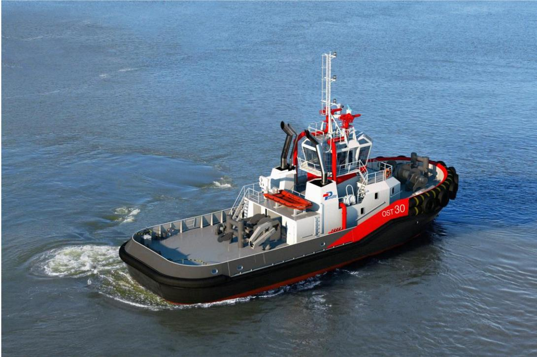
PIRIOU has just recorded a new order for an OST 30 of its tug range dedicated to towage. As the operator of Pointe-à-Pitre harbour in Guadeloupe (French Caribbean island), CARAIBES REMORQUAGE confirmed the construction of a 30.30m tug with 55 tonnes bollard pull and azimuth stern propeller. Built in Vietnam, its delivery is scheduled in the 1st quarter of 2018.
